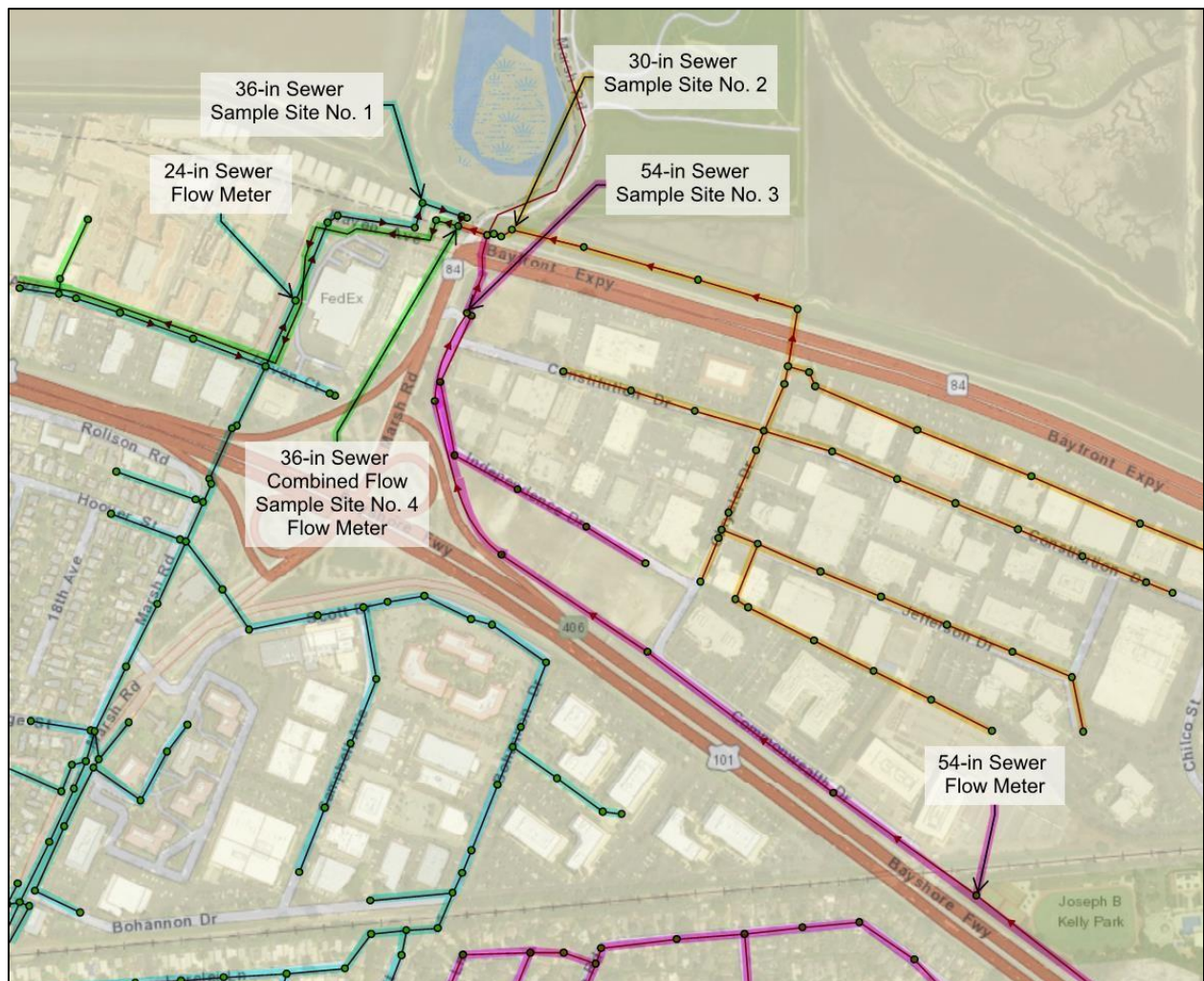
Figure 9: Flow Monitoring and Quality Locations
