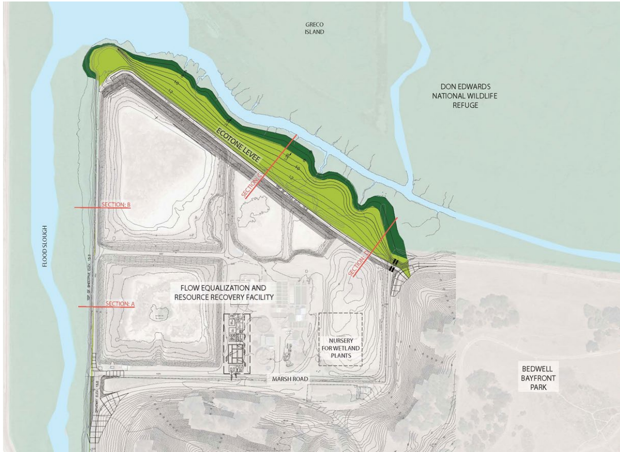
Figure 1 – Levee Improvements Plan View
