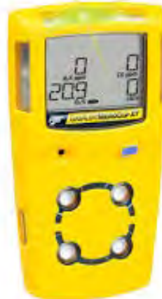
Photo 2-2. Typical Personal Four-Gas Monitor
