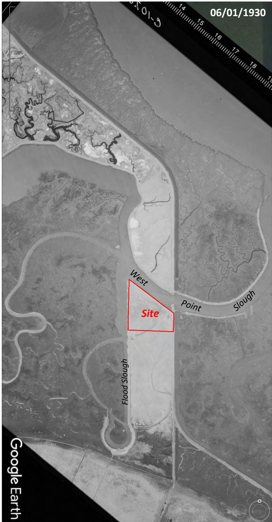
Figure 3. Site location on 1930's aerial photo, Bayfront Recycled Water Facility and Levee Improvements Project. By 1930, drainage improvements included dredging Flood Slough to the bay shore at Marsh Road. West Point Slough appears wider and deeper than seen on current aerial photos, with apparent levee improvements as well.
