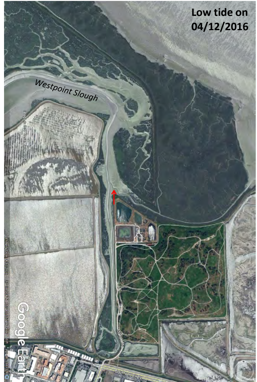
Figure 7. Potential RO Concentrate discharge point to Westpoint Slough, Bayfront Recycled Water Facility and Levee Improvements Project. At high tide, bay waters inundate mudflats and tidal marsh plains in the vicinity of the site. At low tide, Westpoint Slough drain to single-thread channel, exposing mudflats as tidal marshes drain. Synchronizing discharge of RO concentrate with high tide would maximize mixing and circulation to the bay. Red arrow indicates potential discharge location.
