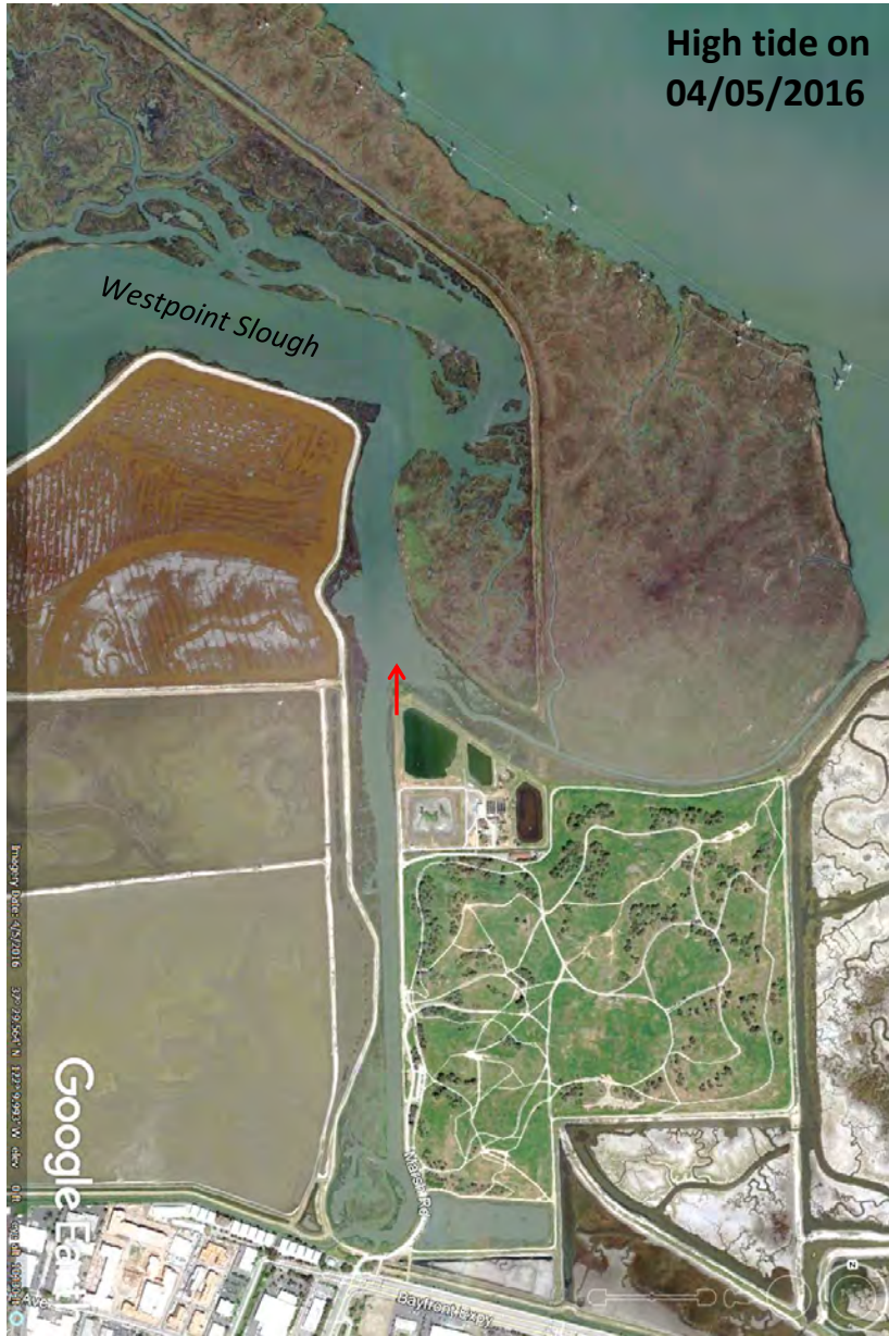
Figure 7. Potential RO Concentrate discharge point to Westpoint Slough, Bayfront Recycled Water Facility and Levee Improvements Project. At high tide, bay waters inundate mudflats and tidal marsh plains in the vicinity of the site. At low tide, Westpoint Slough drain to single-thread channel, exposing mudflats as tidal marshes drain. Synchronizing discharge of RO concentrate with high tide would maximize mixing and circulation to the bay. Red arrow indicates potential discharge location.
