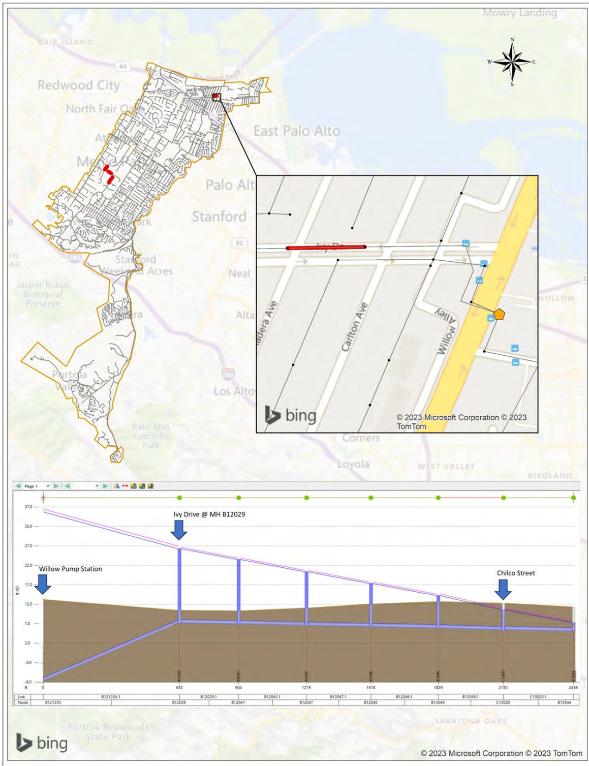
Figure 5.6 Hydraulic Profile after Conversion of the Willow Pump Station Discharge (Ivy Drive) Gravity Sewer to an Extended Force Main
